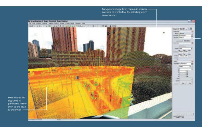
Controls for scan field-ofview, scan, density, traverse workflow and project setup.
