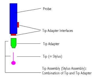
Note that the terms 'Tip' and 'Stylus' are equivalent. The former is used in by the TPI, while the Compensation Application mainly uses the latter.
