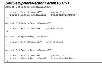
Command structures for setting/getting the sphere region parameters.
