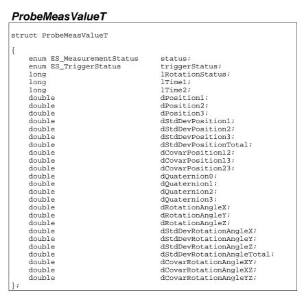
This struct describes a single measurement (6 degrees of freedom) in a 6DoF continuous measurement stream. *Time1* indicates seconds expired since a measurement start. *Time2* indicates microseconds expired within the last second. The total elapsed time in microseconds is:
