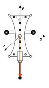
The tip position and probe orientation is returned with respect to the user coordinate system (transformation parameters). The *probe orientation* is described by the rotation angles (xAngle, yAngle, zAngle) or the quaternion (q0, q1, q2, q3). In terms of rotation angles the rotation matrix R is defined as in Section 9.2.4 . In terms of the quaternion it is given by
