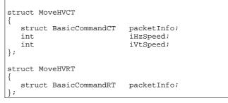
The speed parameters are prefixed with +/-(clockwise is + and anti clockwise is -), to specify the direction of movement.
